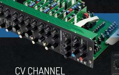
The unique CV-Channel is both, stereo channel and musical instrument. It links professional audio with the modular analogue synth world. It is a stereo channel with VCA technology which allows controlling parameters by hand and by control-voltage (CV) at the same time. CV can be sourced from external equipment or from integrated CV-stages. Composing, sound designing and mixing are brought together by this thoroughly musical approach.
